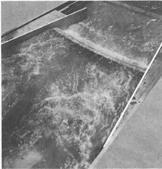
Fig. 18. Pool elev, 800 dischg, 6340 cfs; TW elev, 698.4
