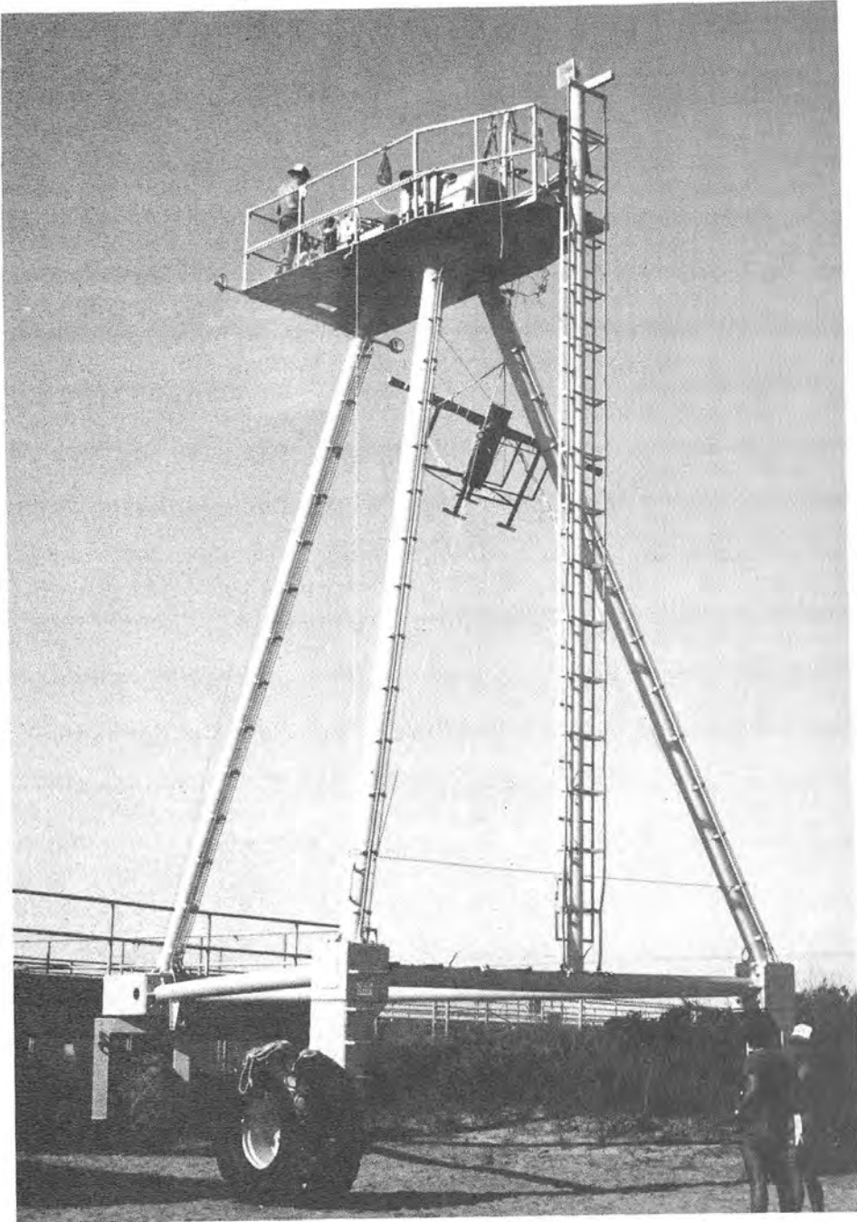
FIGURE VI-3: Preparing for field installation: the DPG suspended underneath the operator's platform of the CRAB.
