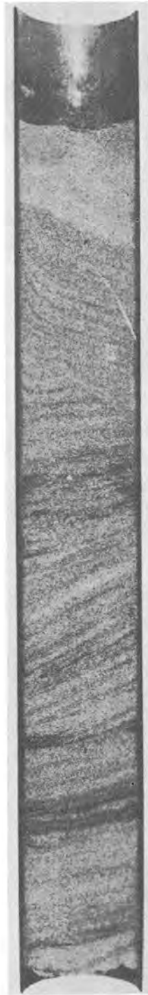
Fig. 19. 3-in.-diameter undisturbed sand sample from depth of 108.5 ft to 110.5 ft. Note that entire sample is highly stratified. Dark strata near bottom of sample contain lignite
