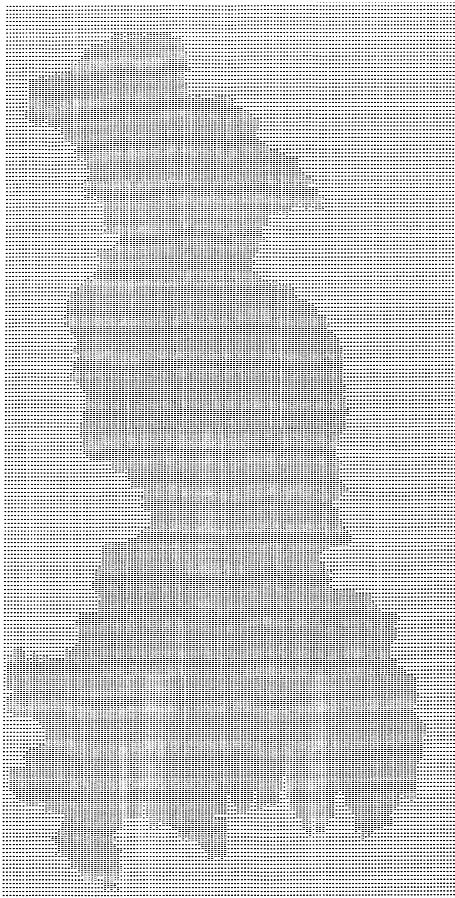
Figure 8. High-speed-printer map of watershed after deletion of islands
