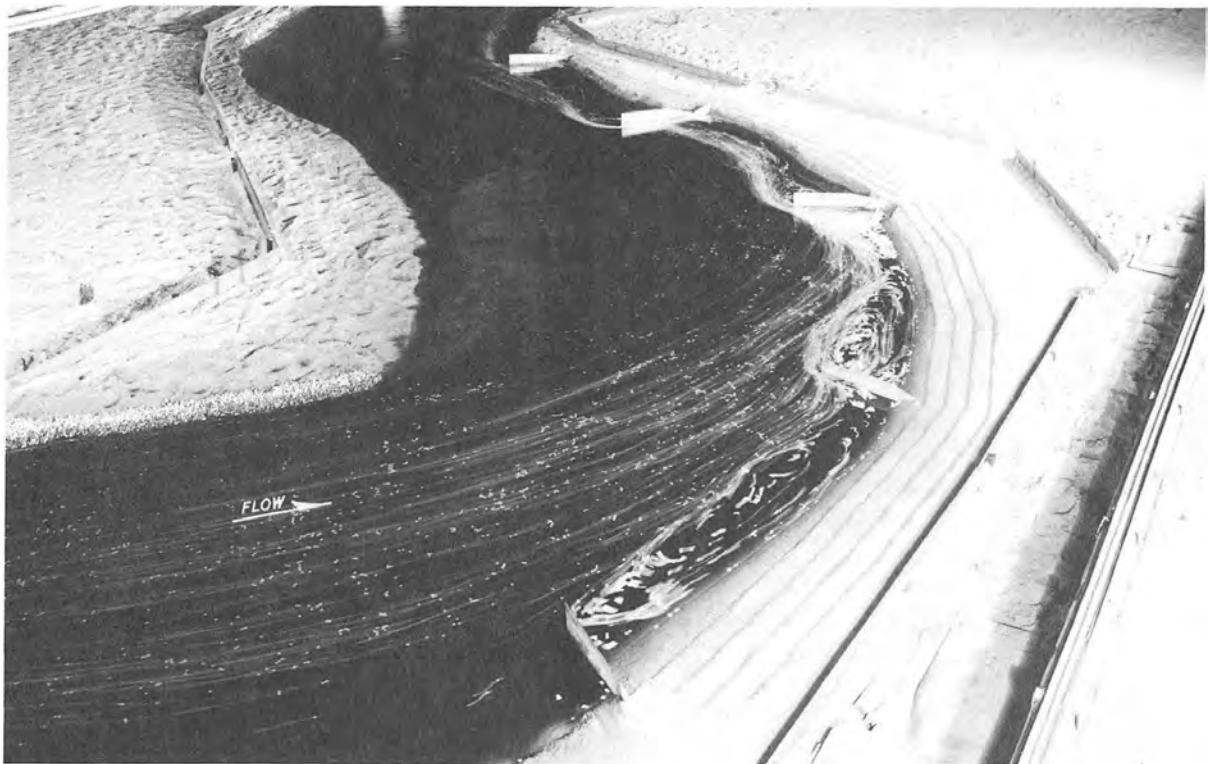
Figure 12. Surface flow patterns; spur dike angle 75 deg
