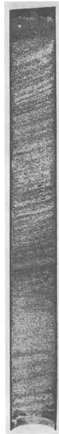
Fig. 20. 3-in.-diameter undisturbed sand sample from depth of 96.5 ft to 99.0 ft. Note discoloration at top of sample caused by intrusion of drilling mud
