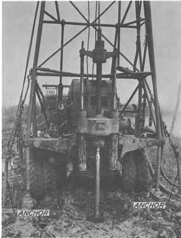
Fig. 7. A typical anchoring arrangement
