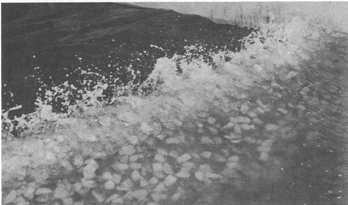
Fig. 7. A 21-ft wave breaking on the complete breakwater -- scale 1:30
