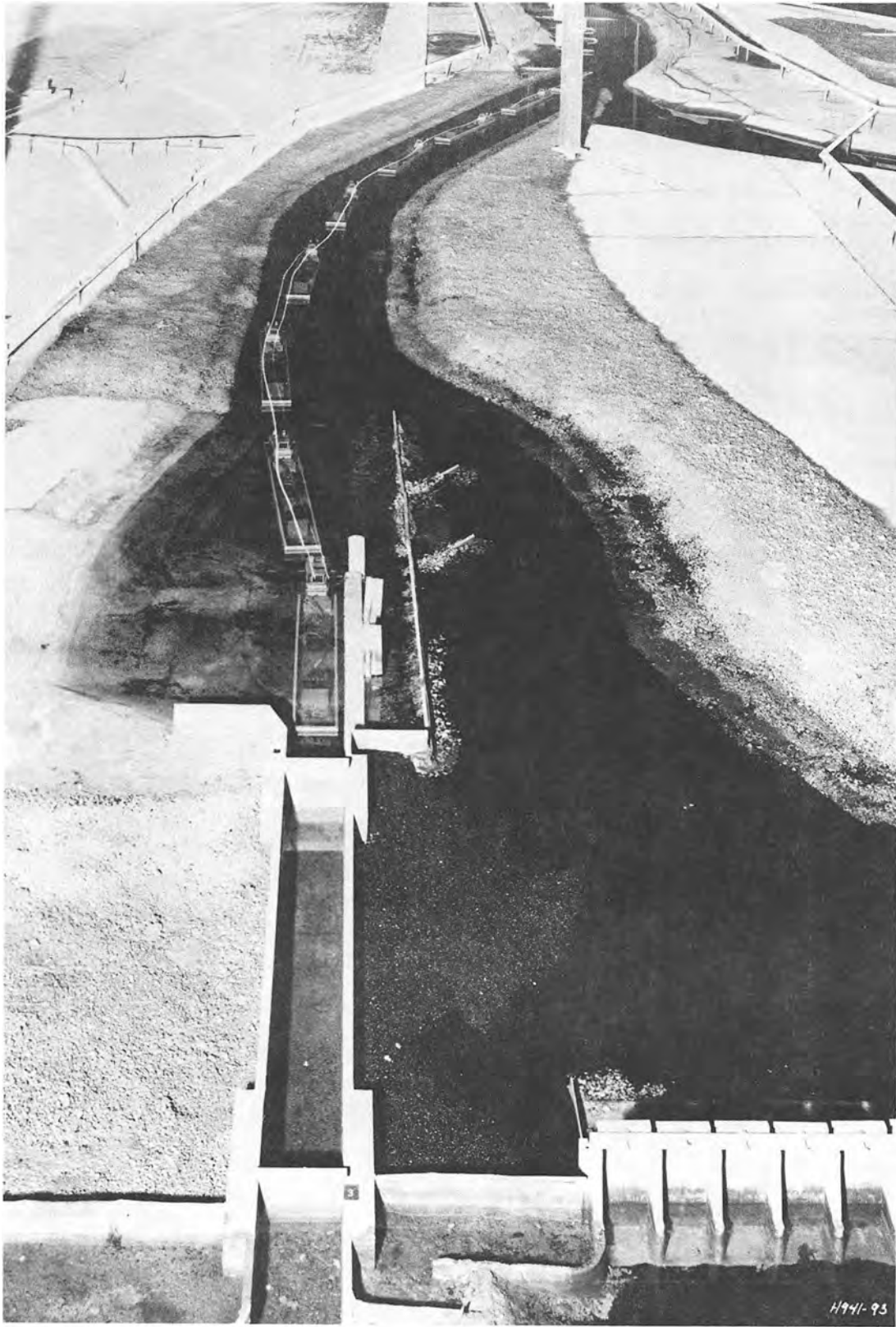
Photo 18. Plan B-35, upbound tow approaching the lock; discharge 31,000 cfs, tailwater el 21.0 (normal)
