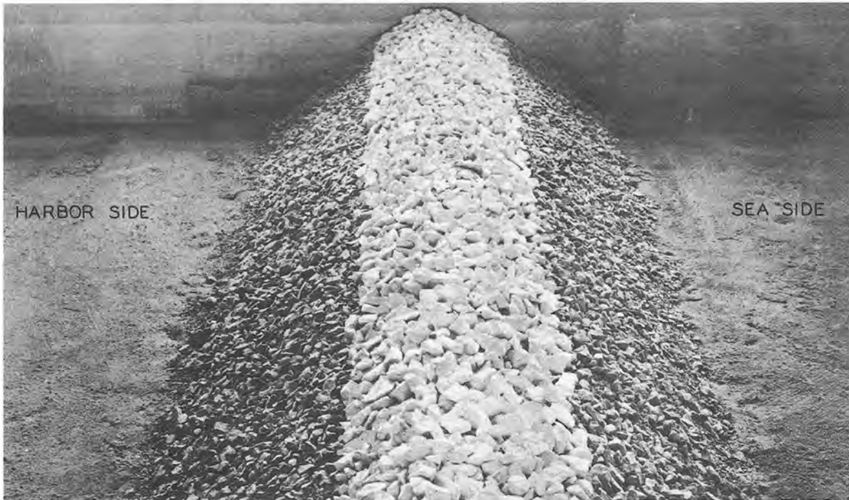
Fig. 6. Complete breakwater section before wave attack -- 1:45-scale model
