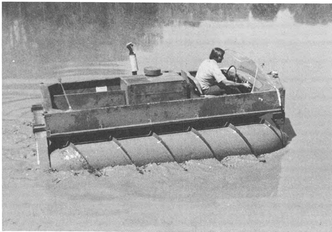
Figure 22. The Marsh Screw, a smaller archimedean screw amphibious craft
