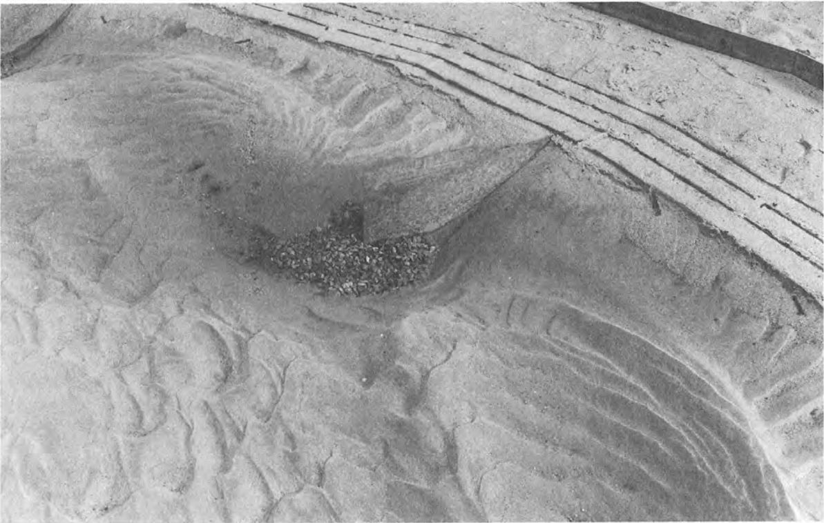
Figure 19. Final conditions for stone apron after 24 hr
