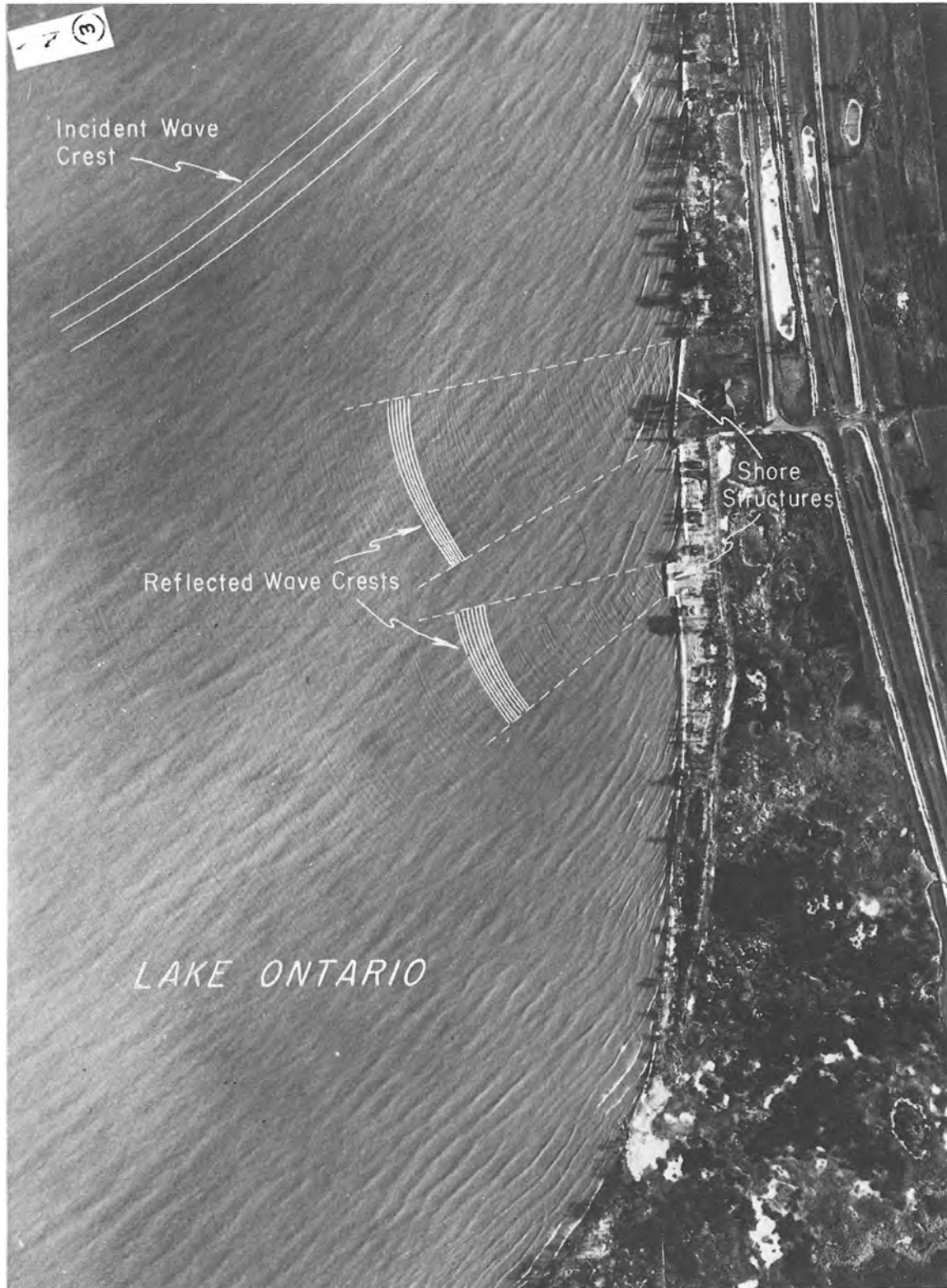
Figure 2-60. Wave Reflection at Hamlin Beach, New York
