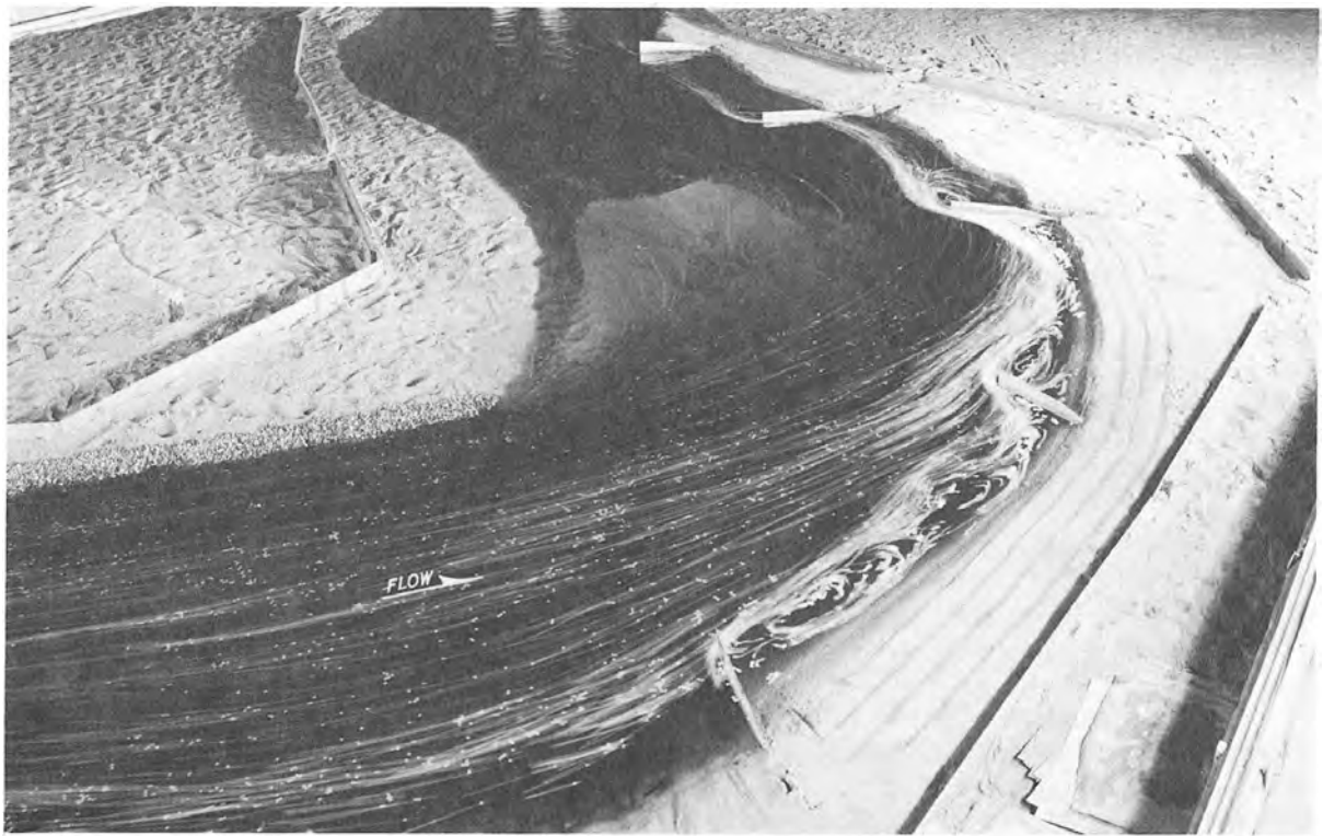
Figure 11. Surface flow patterns; spur dike angle 60 deg
