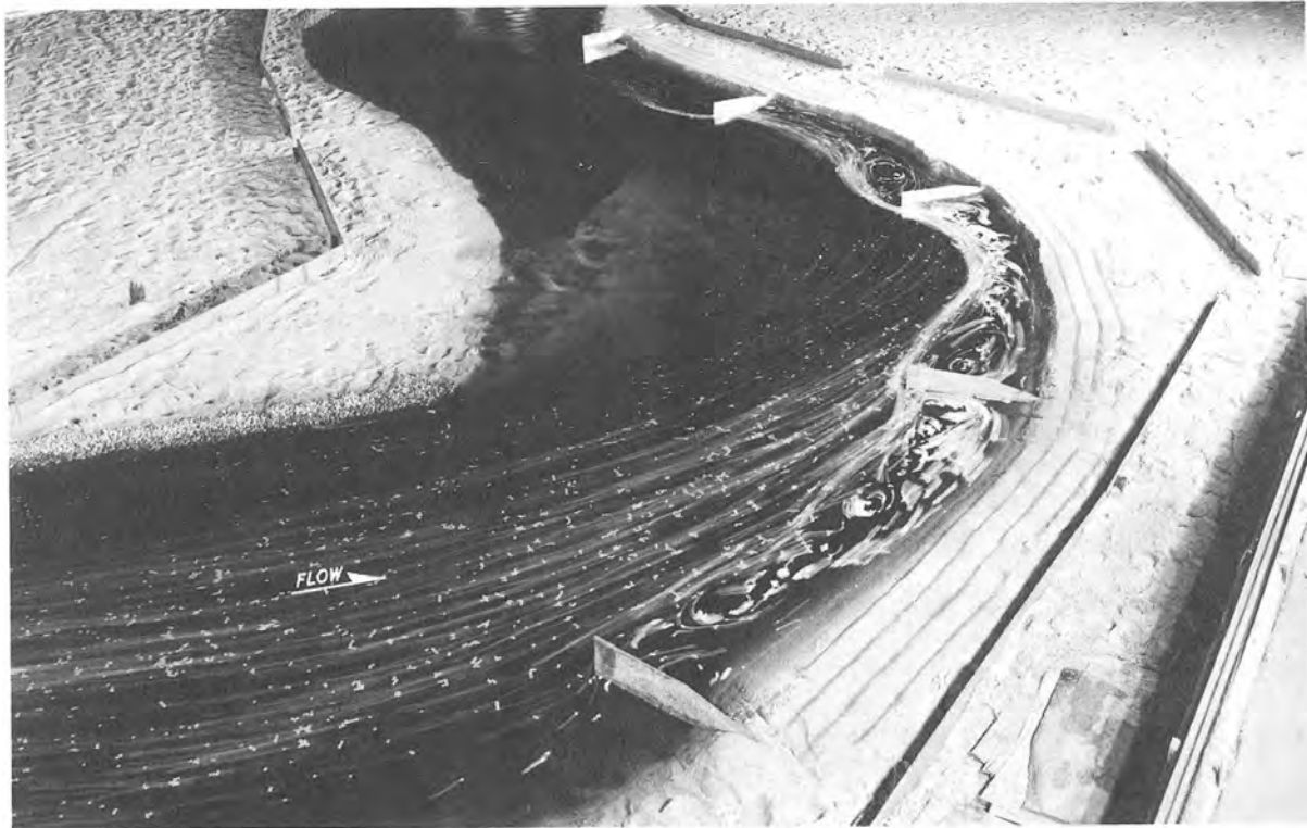
Figure 13. Surface flow patterns; spur dike angle 105 deg
