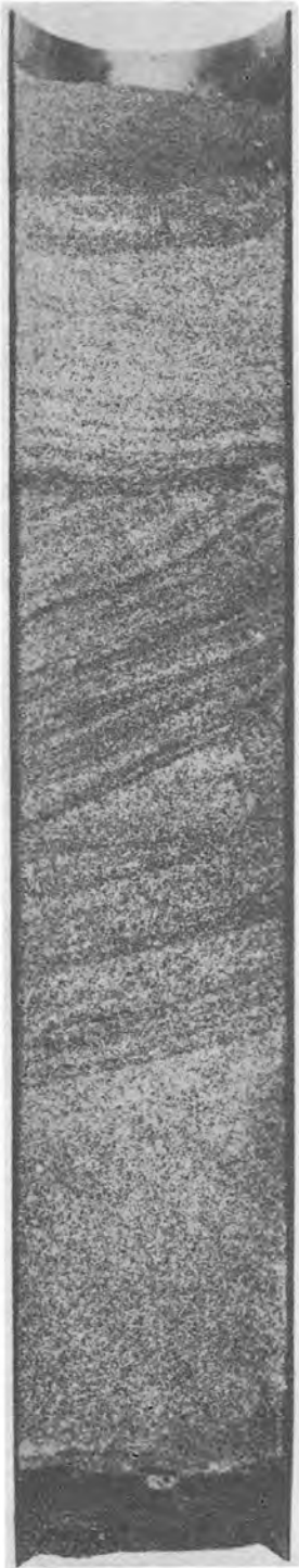
Fig. 18. 5-in.-diameter undisturbed sand sample from depth of 46.5 ft to 48.9 ft. Note discoloration at top of sample caused by intrusion of drilling mud
