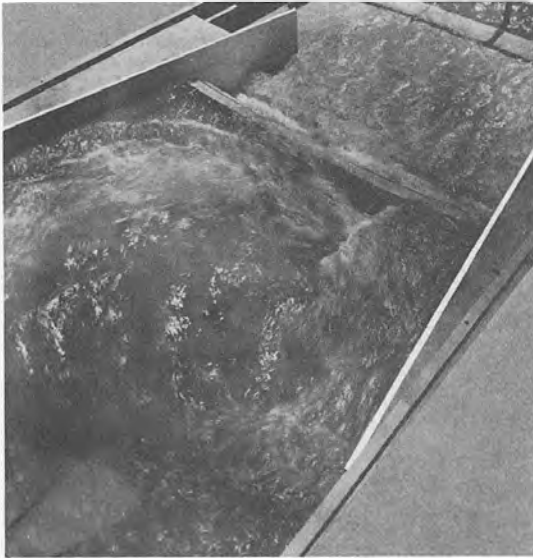
Fig. 16. Pool elev, 800 dischg, 3170 cfs; TW elev, 692.7
