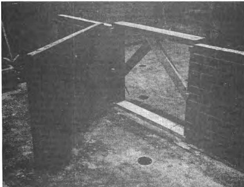
Figure 32. A restraining frame placed between the brick walls from which the closure can be pulled against the walls by springs
